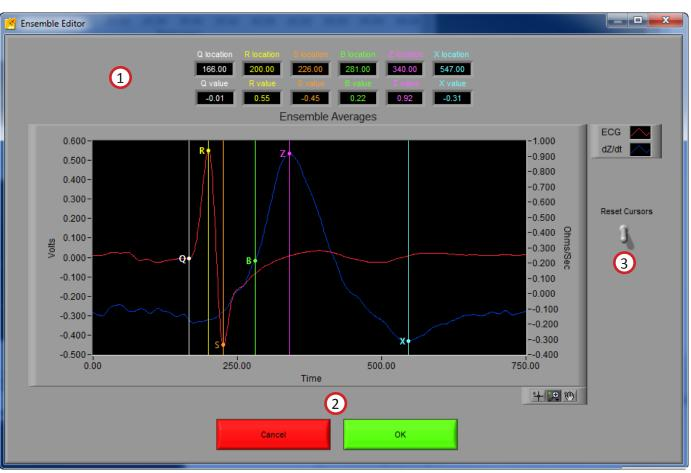
The Systolic Points Editor allows for the calculated placement of P, Q, R, S. T, B, X and Z (1) to be relocated. In order to move the respective landmark, position the mouse over the cursor, depress the left mouse button and drag the cursor to the desired location. After exiting the editor, new values are calculated per the new placement.
