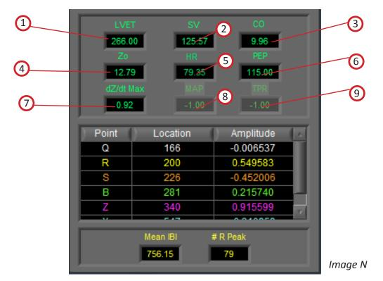
**LVET(1):** The Left Ventricle Ejection Time (LVET) is defined as the distance (in ms) between the X point and B point in dZ/dt. This value will be highlighted red if the X point has been estimated rather than identified.
