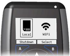
Use the **left and right** arrows to place the selection box over the desired mode. Press the **B** button to select that mode and continue to the configuration screen. The unit will power itself off if left on this screen for more than 5 minutes. To manually shutdown from this screen, press the **A** button.
