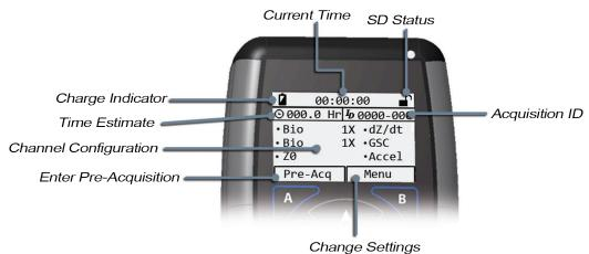
This screen is a summary of relevant information on the acquisition configuration. It is intended to allow you to quickly review the configuration to verify setup before proceeding. The following is a rundown of the key elements.
