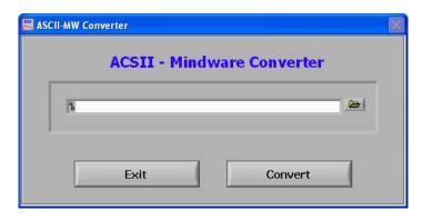
The ASCII-MW Converter allows the conversion of any text file containing data in tab-delimited columns to the .mw format so that it may be used in any analysis application. To begin conversion, select a text file containing data by using the browse button on the file path control and pressing Convert. To exit the converter and return to the setup screen, press Exit.
