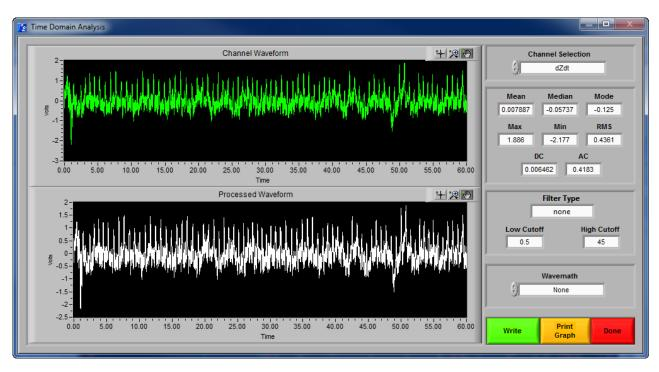
Time domain static analysis allows for various filters and wavemath to be done to the available signals. Two displays are shown on this screen:
