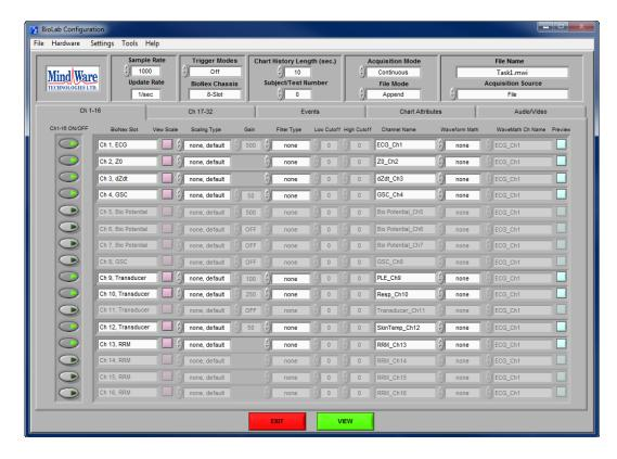
The Channels submenu contains the settings for each channel present in the file. When a MindWare file is first opened, all channels present in the file are enabled for viewing. The following settings are available for each channel in the file:
