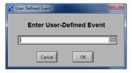
From this window, an event with any definition can be inserted into the file. Previously used event definitions are saved for future use, and accessible from the drop down entry box. Pressing OK inserts the event. Pressing cancel results in the event not being inserted in the file.
