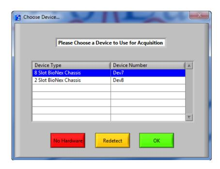
**No Hardware:** This button proceeds to the BioLab Configuration screen without selecting any device listed for use in acquisition.
