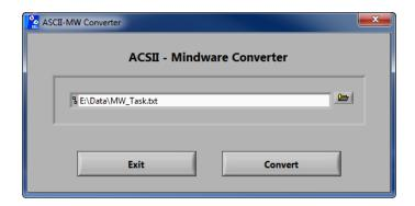
The ASCII-MW Converter allows the conversion of any text file containing data in some character-delimited columns to the .mw format so that it may be used in any analysis application. To begin conversion, select a text file containing data by using the browse button on the file path control and pressing Convert. To exit the converter and return to the setup screen, press Exit.
