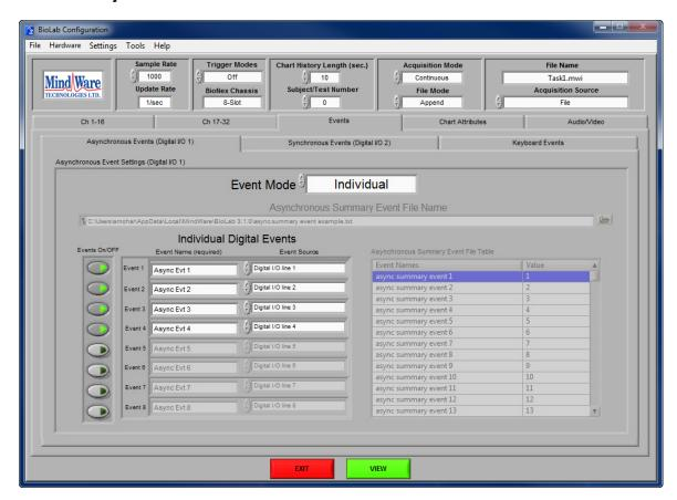
The Asynchronous Events submenu indicates how the asynchronous event channels were configured when the file was acquired. This submenu is merely a display and is **not** editable, as changes made here will have no affect on the file playback (since asynchronous event channels are not saved in the MindWare file).
