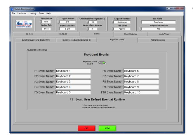
The Keyboard Events submenu contains settings for configuring the keyboard events available to the user during file playback. The settings are initialized to the keyboard event names at the time of acquisition of the current MindWare file. The following settings are available:
