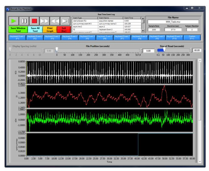
The BioLab File Playback screen is the main file viewing window where file playback can be controlled and post-acquisition event editing can be performed.
