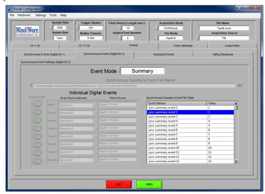
The Synchronous Events submenu contains options for configuring the display of synchronous digital event channels present in the MindWare file. The following settings are available:
