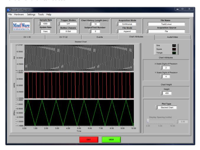
The Chart Attributes submenu contains settings for adjusting how the data is displayed on the File Viewer screen, and behaves the same as it did in acquisition mode (see **Section 2: BioLab Configuration**). The settings are initialized to how they were set that the time of acquisition of the MindWare file, but are fully adjustable in file playback mode.
