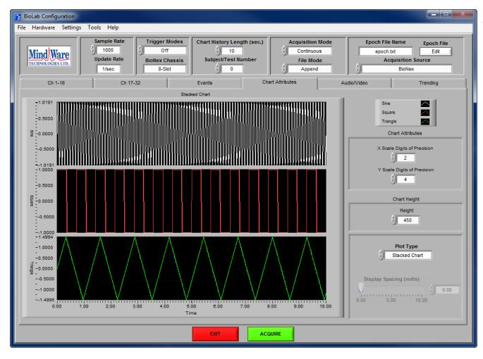
The Chart Attributes submenu contains settings for adjusting how the data is displayed on the Acquisition screen. The following settings are available:
