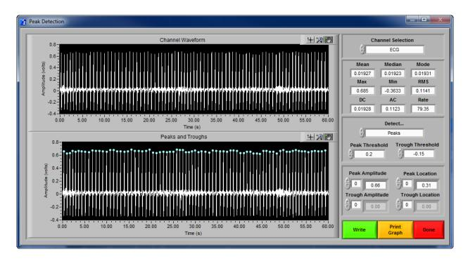
The Peak Detection window allows for peaks and troughs of the specified waveform to be detected and labeled. There are two display plots shown:
