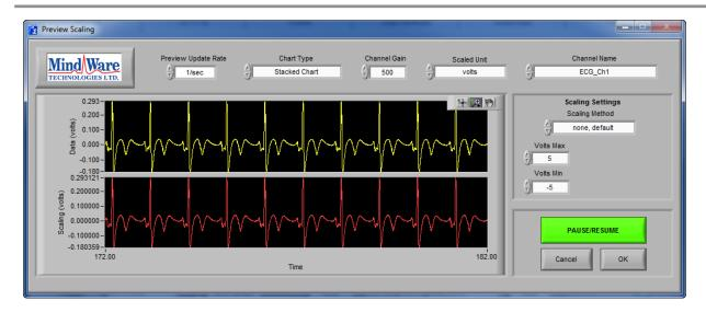
The Preview Scaling screen is used to see how various scaling methods can affect the channel to which they are being applied. The following settings are available:
