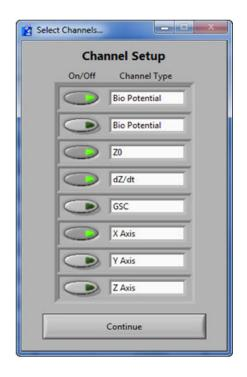
From this screen the user can specify which channels will be used for acquisition. Up to four channels can be selected simultaneously. If any more than 4 channels are selected, a warning will appear and the most recently selected channel will be automatically deselected. When all desired channels have been enabled, press **Continue** to return to the Network Device Detection screen.
