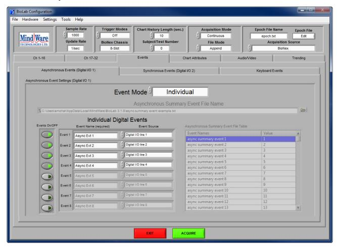
The Asynchronous Events submenu contains setup options for configuring the asynchronous digital I/O on the BioNex. Asynchronous events are sampled at ~500 samples per second, and are not guaranteed to be in sync with the acquired data. The signals enabled in this submenu are not displayed on the Acquisition screen or saved in the MindWare file, but events detected on these lines will appear in the associated Event file.
