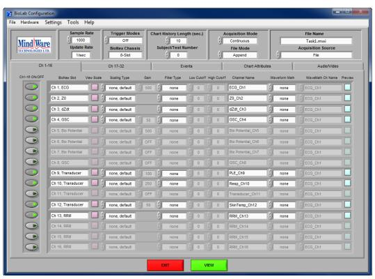
When a MindWare file is opened, it is loaded into the BioLab Configuration screen with all of the settings as they were set at the time of the file's recording. All channels which are present in the file are automatically enabled. Also, notice that the button which read "Acquire" has changed to "View". Once again, the configuration screen is divided into three sections: Menu Bar Settings, Main Settings, and Sub Menu Settings.
