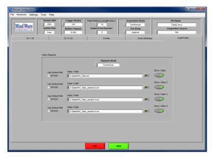
**Use Default Path:** When checked, the video file with the expected name will be loaded and played back. Uncheck this box to custom map a video file for playback.
