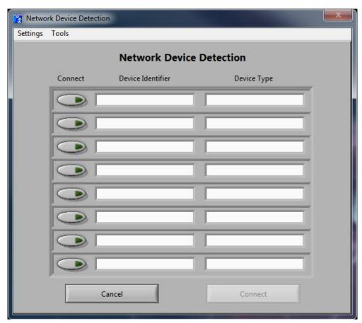
As network devices attempt to connect to the system, they will appear in the table on this window. Up to 8 network devices can be listed simultaneously. The following settings are available from the Settings menu:
