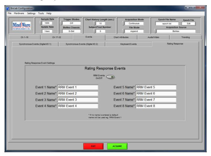
The Rating Response submenu contains settings for configuring the events obtained from Rating Response modules in the system. This submenu will only be available when using a newer model 8-slot BioNex. Rating Response events are captured asynchronously, and up to 8 unique events can be captured (2 per channel).
