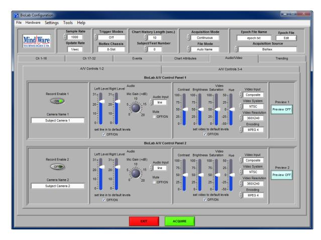
The Audio/Video submenu contains settings for the acquisition of up to 4 A/V streams from the MindWare Video ACQ modules. These settings are only adjustable when 1 or more of these modules are present in the system.
