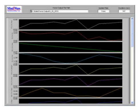
The Trending screen appears during acquisition if at least one trend was enabled on the Trending submenu of the BioLab Configuration screen. The trends are shown in a stacked plot display, with each plot having its own unique y-axis (amplitude) but sharing its x-axis (time) with all other trends. Each trend is labeled along its y-axis with the Trend Tag specified on the BioLab Configuration screen. The graph palette is located in the lower left hand corner.
