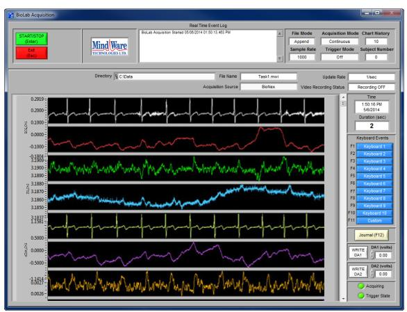
In the upper left corner of the screen are the acquisition controls. When in Continuous acquisition mode, following controls are available which control the acquisition:
