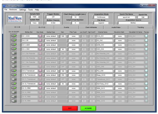
**On/Off:** This control enables/disables the specified channel for acquisition. In order for the channel to be enabled, there must be a module in the corresponding slot. *Note: Channel On/Off is disabled when collecting from network devices.*
