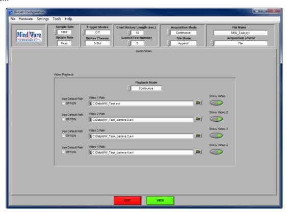
Only the Audio/Video submenu is available when a video file is opened for playback. All videos associated with the selected video file are automatically mapped and enabled for playback. This submenu behaves in the same way as in File Playback mode, with the exception that the **Playback Mode** control is fixed to continuous mode.
