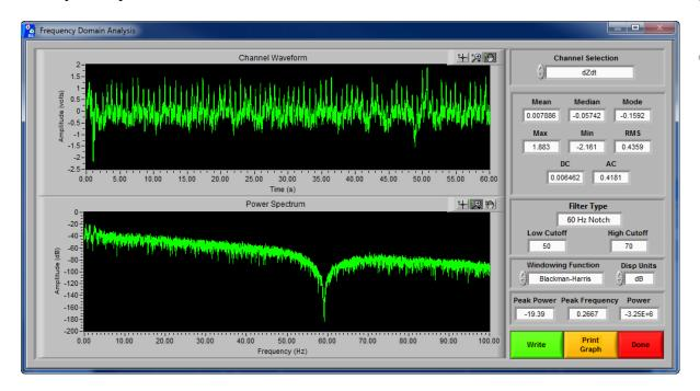
Frequency domain static analysis allows for various filters to be applied to a signal after applying an FFT (Fourier Fast Transform) to the specified channel waveform. This is very useful in determining the effect of noise on different frequency bands on the original signal. There are two display plots shown:
