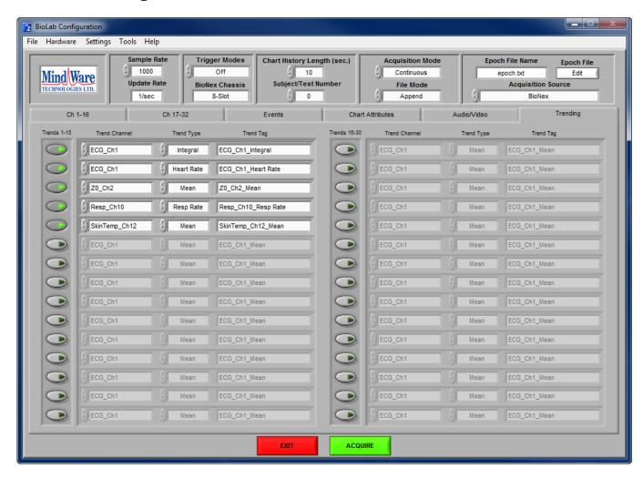
The Trending submenu contains settings for specifying trends to be calculated during acquisition. Trends are basic statistical calculations that are graphed and output to a file real time alongside the standard data acquisition. Up to 30 trends can be computed and displayed simultaneously, and can be applied to any channel enabled for acquisition. The following settings are available:
